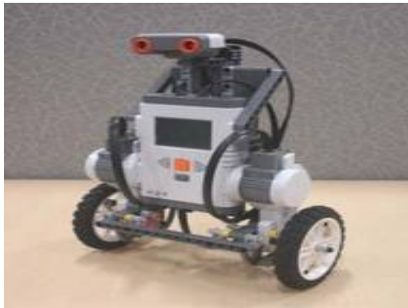
Fig.1 Inverted Pendulum based two-wheeled self -balancing Robot
